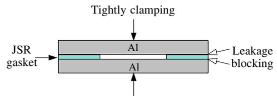
**Fig. 5** Schematic illustration of the gasket inserting scheme
