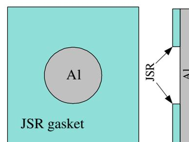
**Fig. 6** Spin-coated and photolithographic patterned JSR gasket
