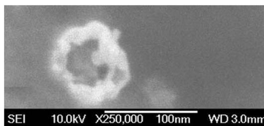
**Fig. 4** Cryo FEGSEM photomicrograph of preformed silver nanoring before the addition of NaBH<sub>4</sub>
