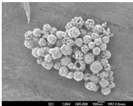
**Fig. 3** FEGSEM photomicrograph of silver spherical hollows suspension obtained at  $25 \pm 0.5$  °C
