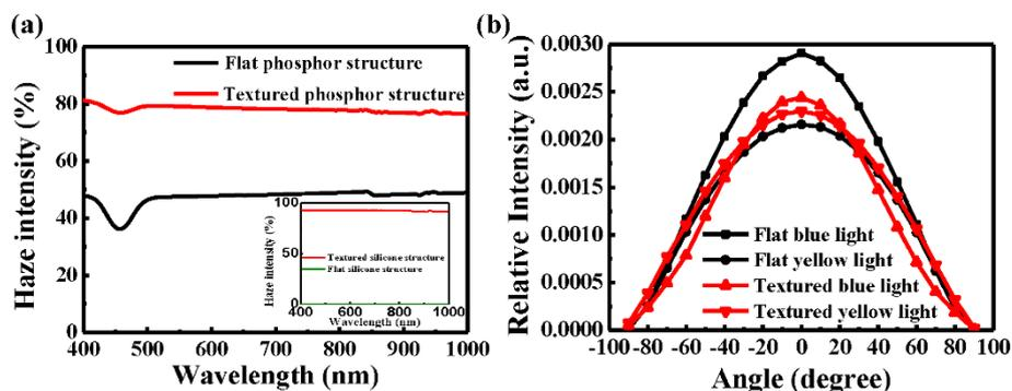
**Figure 3 Wavelength-dependent haze intensity and angular-dependent relative intensity measurements.** (a) The measured wavelength-dependent haze intensity with phosphor in flat/textured silicone structures; the inset is the flat/textured silicone structures without phosphor, and (b) measured angular-dependent relative intensity of the flat and textured phosphor structures at a driving current of 120 mA.
