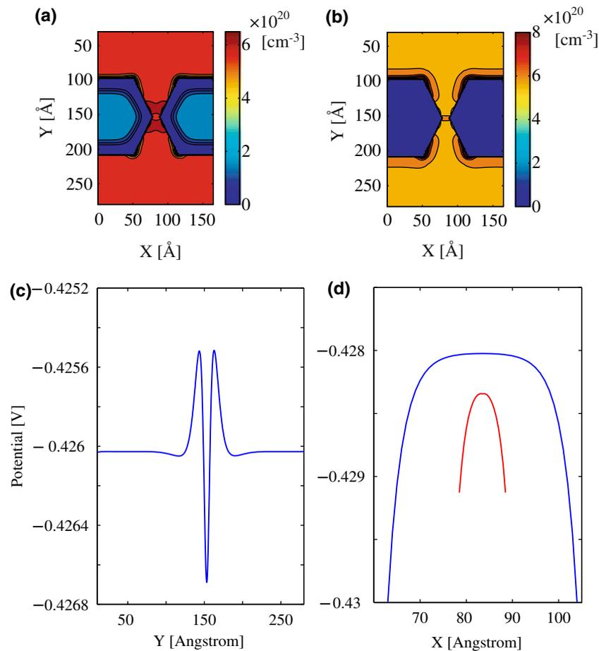
**Fig. 2** (a) and (b) Contour plot of ion concentration in the electrolyte and mobile charges in the membrane for a surface charge of  $-0.064 \text{ C m}^{-2}$ , a doping concentration  $N_d^+ = 2 \times 10^{20} \text{ cm}^{-3}$  and an ion concentration of 1 M: (a) anion and
