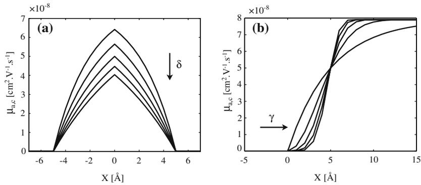
**Fig. 3** Mobility profiles at different positions in the channel: (a) along the center plane of the device  $Y_c$  for different  $\delta$  varying by unitary step from  $\delta = 3 \text{ \AA}$  to  $\delta = 7 \text{ \AA}$  and  $\gamma = 1$  (b) along  $Y_1$  near the wall for  $\gamma$  varying by unitary step from  $\gamma = 1$  to  $\gamma = 5$  and  $\delta = 5$
