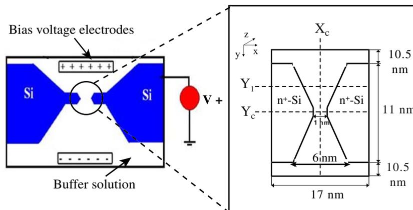
**Fig. 1** Schematic of the device geometry:  $xy$  cross-section through the center of the device. The drawing is not to scale
