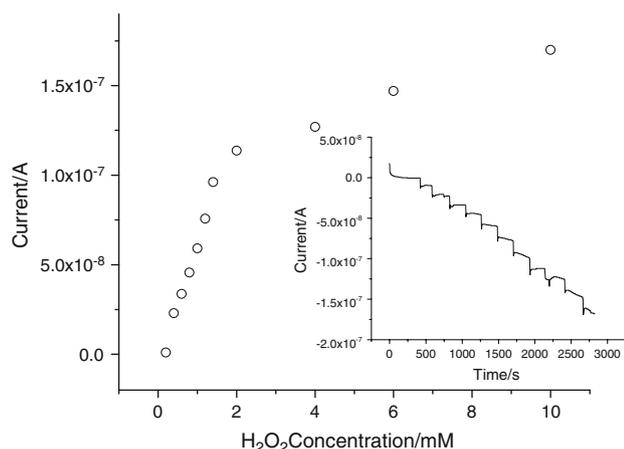
**Fig. 4** Calibration curve for the determination of  $\text{H}_2\text{O}_2$  at the polyaniline/gold nanocomposite electrode. Applied potential:  $-400$  mV, supporting electrolyte: 0.1 M pH 7.0 PBS with  $\text{N}_2$ -saturated. Inset: typical steady-state response of the biosensor on successive injection of  $\text{H}_2\text{O}_2$  into stirring PBS
