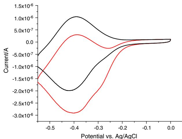
**Fig. 3** Cyclic voltammograms of polyaniline/gold nanocomposite electrode in 0.1 M PBS (pH 7.0) without and with 1 mM  $\text{H}_2\text{O}_2$  concentration at 20 mVs. In the absence of  $\text{H}_2\text{O}_2$ , a pair of the redox peaks of MP-11 was observed, the voltammetric behavior changes drastically in the presence of  $\text{H}_2\text{O}_2$
