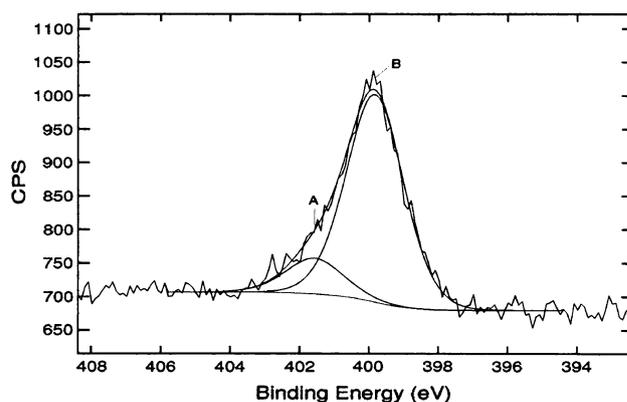
**Fig. 2** The X-ray photoelectron spectra of the N 1s for the polyaniline/gold nanocomposite. The peak A at binding energy of 399.4 eV corresponds to the benzenoid amine ( $-\text{NH}-$ ). A higher binding energy peak (Peak B) centered at 401.2 eV is also found in Au-Polyaniline
