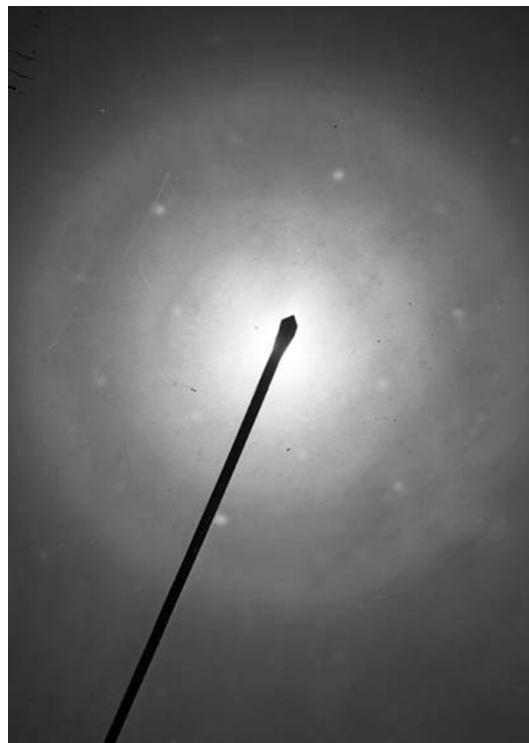
Fig. 2 ED of Fe 2 O 3 /CP(St–OA) nanoparticles
