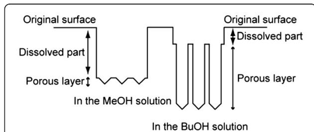
**Figure 5** A schematic of different dissolution modes. A schematic cross-sectional view illustrating porous layers anodized in the MeOH and BuOH solutions.
