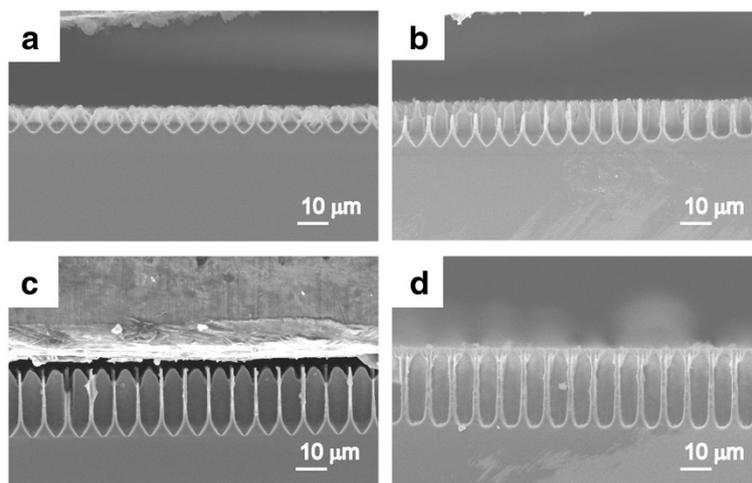
**Figure 1** SEM micrographs of macropores formed in HF solutions containing various types of alcohol. Cross-sectional views of silicon anodized in a 10–20  $\Omega\text{cm}$  prepatterned p-type silicon at  $14 \text{ mA cm}^{-2}$  for 1 h in HF solutions containing (a) MeOH, (b) EtOH, (c) PrOH, and (d) BuOH.
