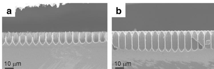
**Figure 4** Comparison of SEM micrographs of macropores formed in HF solutions with and without Et<sub>2</sub>O. Cross-sectional views of porous layers anodized in a 10–20 Ωcm prepatterned p-type silicon at 14 mAcm<sup>-2</sup> for 1 h in (a) HF:H<sub>2</sub>O:EtOH with a composition of 5:6:29 and (b) HF:H<sub>2</sub>O:EtOH:Et<sub>2</sub>O with a composition of 5:6:15:14 in volume.
