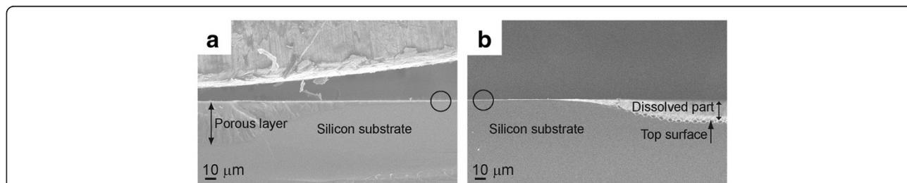
**Figure 3 SEM micrographs of macropores prepared in the MeOH solutions with different HF concentrations.** Cross-sectional views of porous layers anodized in 10–20 Ωcm prepatterned p-type silicon at  $14 \text{ mA cm}^{-2}$  for 1 h in HF: H<sub>2</sub>O:MeOH (a) 22:6:12 (ca. 30 wt.% HF) and (b) 5:6:29 (ca. 8 wt.% HF) in volume. Circles show the positions that have not undergone anodization.
