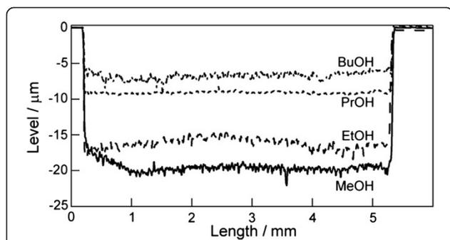
**Figure 2 Topographic profiles.** Cross-sectional profiles of silicon anodized in low-concentration HF solutions with MeOH, EtOH, PrOH, and BuOH.
