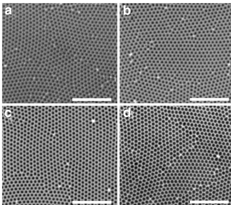
**Figure 1** Set of ESEM top view images of NAA samples (scale bar = 1  $\mu\text{m}$ ). (a) R-OSC(1) ( $L_p = 5 \mu\text{m}$ , and  $d_p = 30 \text{ nm}$ ). (b) R-OSC(2) ( $L_p = 5 \mu\text{m}$ , and  $d_p = 41 \text{ nm}$ ). (c) R-OSC(3) ( $L_p = 5 \mu\text{m}$ , and  $d_p = 52 \text{ nm}$ ). (d) R-OSC(4) ( $L_p = 5 \mu\text{m}$ , and  $d_p = 71 \text{ nm}$ ).
