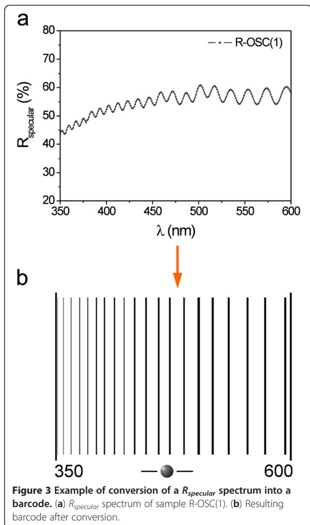
**Figure 3** Example of conversion of a  $R_{\text{specular}}$  spectrum into a barcode. (a)  $R_{\text{specular}}$  spectrum of sample R-OSC(1). (b) Resulting barcode after conversion.
