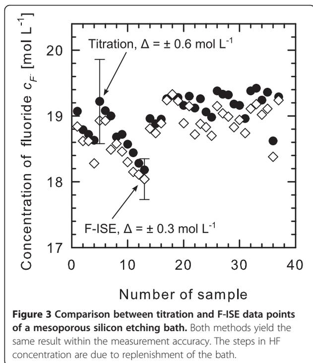
etching. The addition of surface wetting agents reduces the surface tension of the electrolyte, leading to a higher detachability of hydrogen bubbles [13]. Ethanol can serve as a surface wetting agent, as can acetic acid. A crucial factor for the evaluation of a suitable technique is the analysis method's capability of resistance against the aggressive HF.
