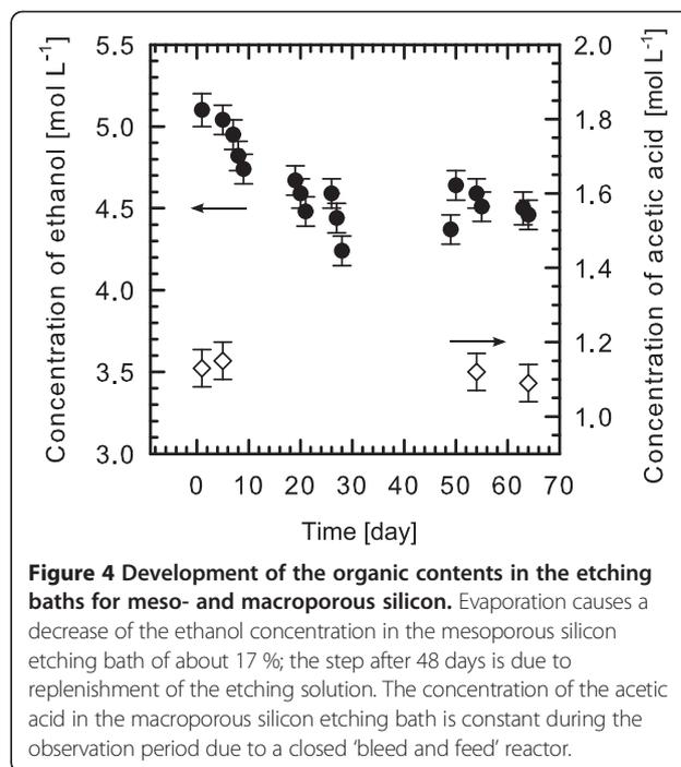
concentration due to evaporation. The reactor for mesoporous silicon is not closed as HF and ethanol may form an explosive mixture. Hence, evaporation cannot be avoided completely. The step in the concentration of ethanol after 48 days in Figure 4 is due to replenishment of the etching solution.
