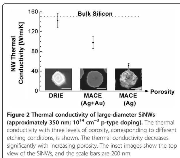
**Figure 2 Thermal conductivity of large-diameter SiNWs (approximately 350 nm;  $10^{14} \text{ cm}^{-3}$  p-type doping).** The thermal conductivity with three levels of porosity, corresponding to different etching conditions, is shown. The thermal conductivity decreases significantly with increasing porosity. The inset images show the top view of the SiNWs, and the scale bars are 200 nm.
