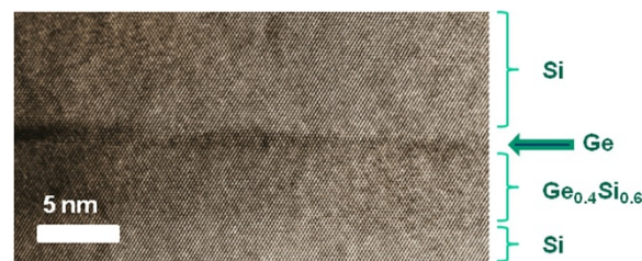
Figure 6 High-resolution TEM image of Ge quantum dots ( d_{\text{Ge}} = 0.3 nm) on 5-nm-thick Ge 0.4 Si 0.6 at 500°C.
