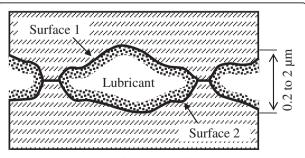
Figure 2 Closed volumes formed by valleys between peaks on contacting surfaces.
