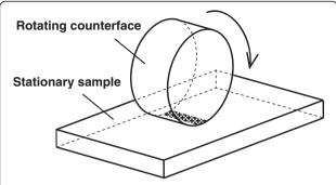
Figure 1 A sliding tribosystem model: cylindrical roller rotating over the motionless block.
