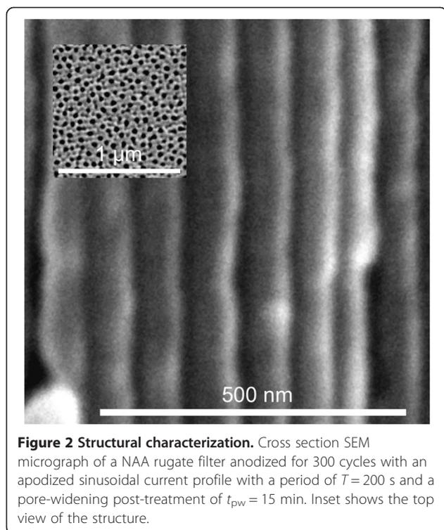
**Figure 2 Structural characterization.** Cross section SEM micrograph of a NAA rugate filter anodized for 300 cycles with an apodized sinusoidal current profile with a period of  $T = 200$  s and a pore-widening post-treatment of  $t_{pw} = 15$  min. Inset shows the top view of the structure.
