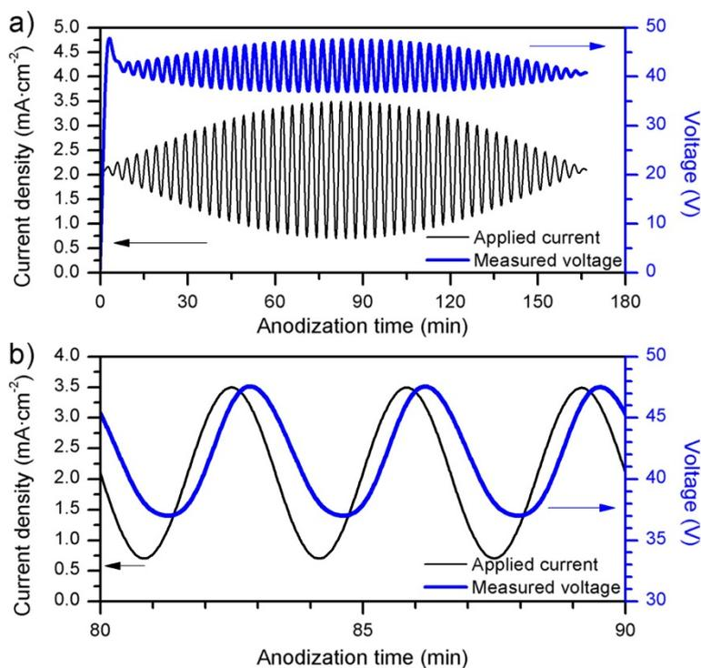
**Figure 1** Characteristic current and voltage evolution during the fabrication of an apodized NAA rugate filter. (a) Full experiment and (b) magnification of the region with maximum amplitude of current profile.
