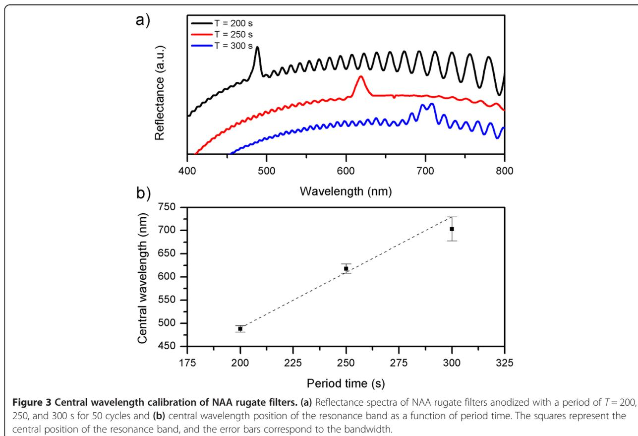
**Figure 3 Central wavelength calibration of NAA rugate filters.** (a) Reflectance spectra of NAA rugate filters anodized with a period of  $T = 200$ , 250, and 300 s for 50 cycles and (b) central wavelength position of the resonance band as a function of period time. The squares represent the central position of the resonance band, and the error bars correspond to the bandwidth.
