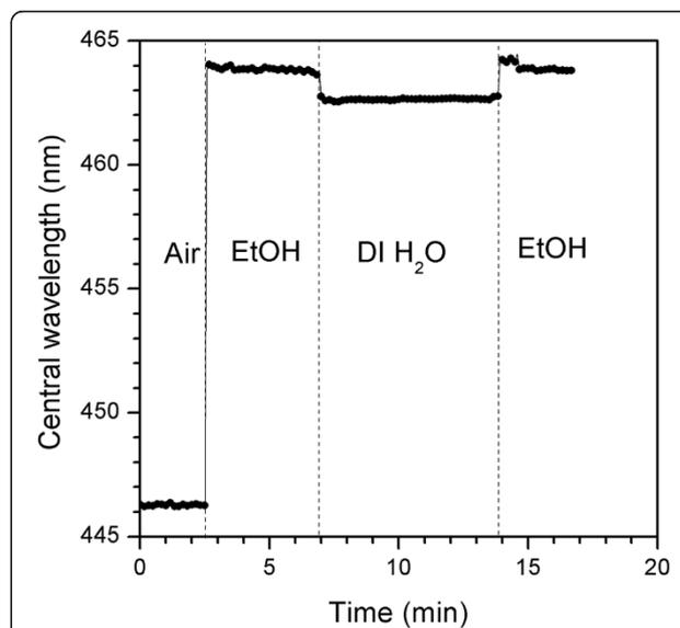
**Figure 5** Sensing results. Real-time measurement of a NAA rugate filter in a flow-cell where EtOH, deionized water, and EtOH were serially flushed in to the chamber.
