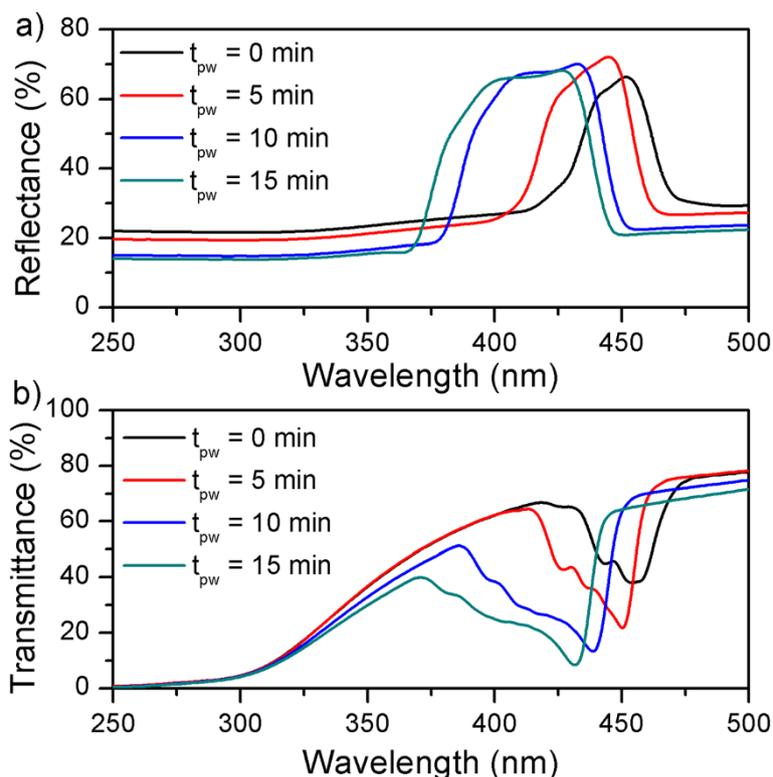
**Figure 4** Reflectance and transmittance characterization of the NAA rugate filters. (a) Reflectance and (b) transmittance spectra of NAA rugate filters anodized for 300 cycles, with an apodized sinusoidal current profile with a period time of  $T = 200$  s.
