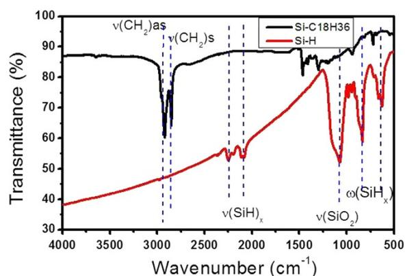
**Figure 2** FTIR analysis of Si NPs before and after functionalization. Si-C<sub>18</sub>H<sub>37</sub> means Si NPs functionalized by the C<sub>18</sub>H<sub>37</sub> group (black curve), and Si-H means Si NPs without any chemical modification (red curve).
